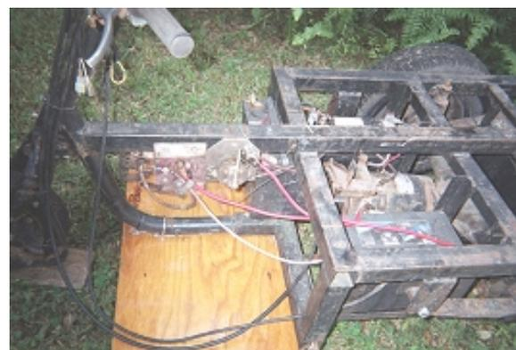
If you don't have facilities or the ability to weld, then you can save a lot of money by just cutting the steel to length and getting it ready for a welder to do the job for you without wasting time. Just check that everything fits together well with the transaxle, front end, battery shapes, etc. before taking it all to be welded. It cost me just \$27 for the steel, and I bartered with a friend for the welding, so the new chassis was almost free!
