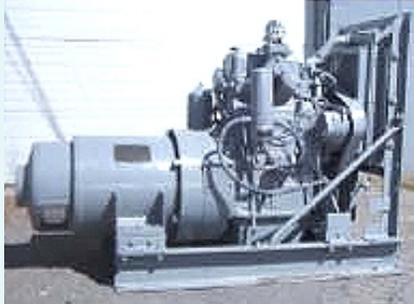
This is the heaviest duty 12.5 kW generator ever built combining the 2-71 Detroit Diesel engine with extremely heavy duty Delco or Emerson brushless alternators. The alternators are all copper wound and usually load test at over 15-20 kW. The 2-71 diesel is the best engine because of its simple design, extremely heavy duty construction, reliability, low 1200 RPM, parts available worldwide, and because it is easy and inexpensive to work on and rebuild.
