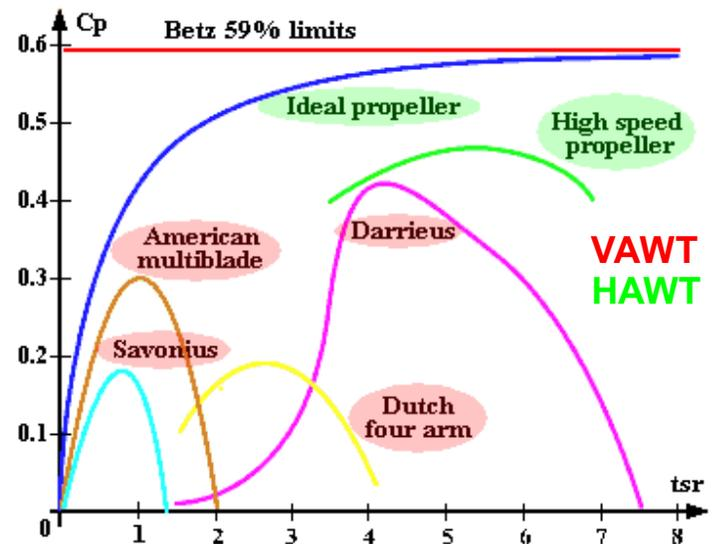
This diagram shows the maximum  $C_p$  theoretically possible, versus Tip Speed Ratio, for different wind turbine designs. Courtesy of <http://www.windturbine-analysis.com/> (Note: used without permission - email address on website no longer valid)
