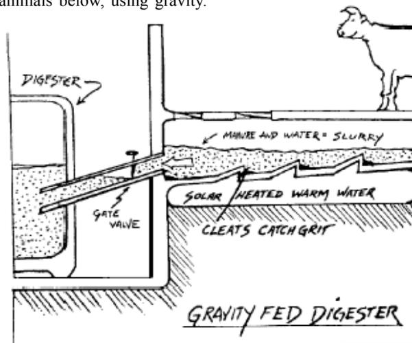
The more that gravity can be utilized for tasks the better. The animal walks around. It can walk up as well as down. If the housing for the animals can be above the digester, then this saves work.
