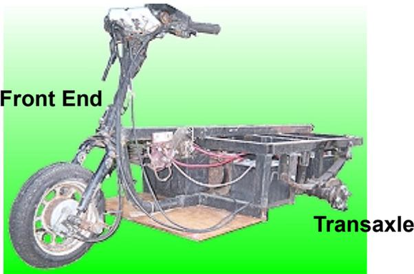
All you need then is to find a MC front end that will work at the higher speeds you will be going. Most front ends from anything bigger than a 150cc motorcycle will work. Before you lay down your money, make sure the assembly has a good tire, brakes and speedo, and that the suspension is in good shape.
