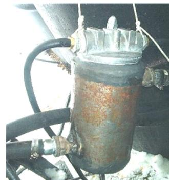
Water fittings were then welded to the sides. Engine coolant was run through this homemade water jacket.
