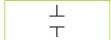
2 Normally open (Form A) contact schematic.
